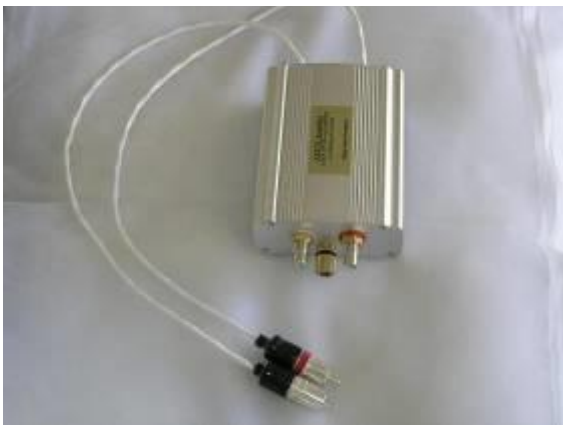
NEXUS : STEP-UP TRANSFORMER
